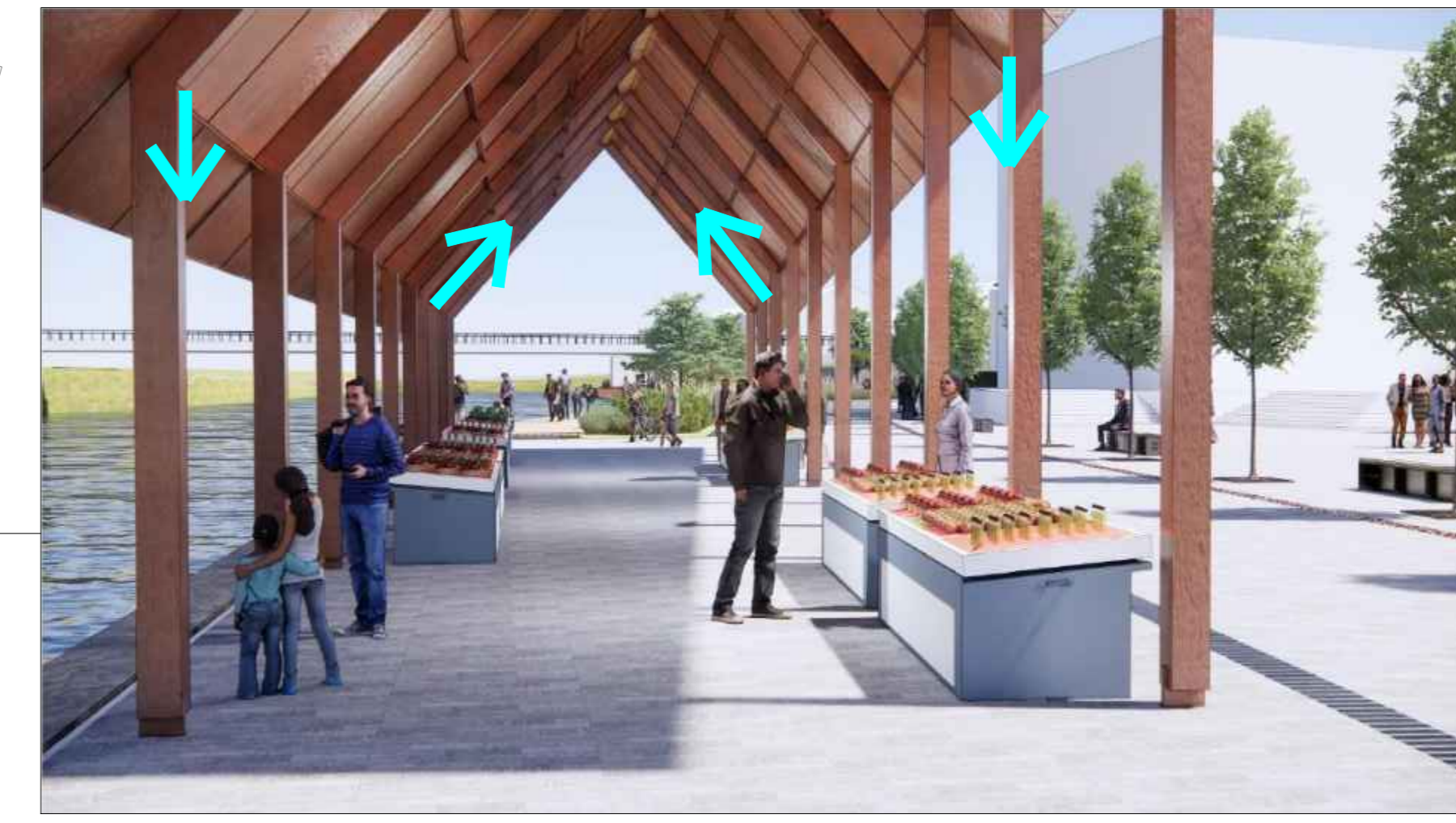
FEATURE LIGHTING - SCHREDER VALINTA LED SPOT LIGHT MOUNTED ON RIVER FRONT ROOF SUPPORT STRUCTURE TO HIGHLIGHT THE EAVES AND INTERNAL SPACE. EAVES TO BE ILLUMINATED BY PHOTOCELL. DOWNWARD SPOTS TO HAVE LIGHTING CONTROL SWITCH FOR WHEN SPACE IS USED FOR EVENTS.
