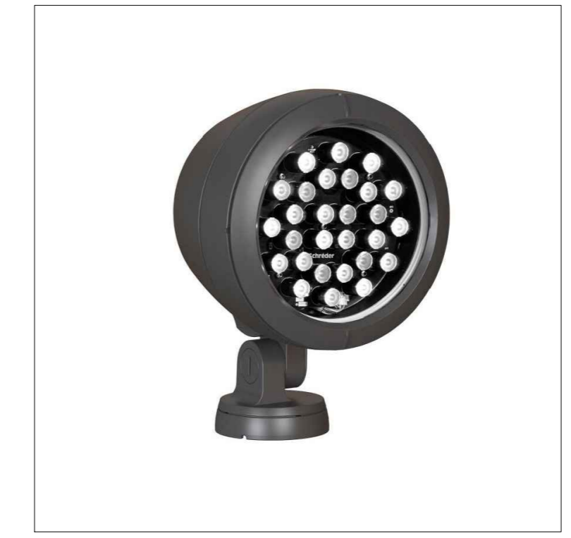
FEATURE LIGHTING - SCHREDER VALINTA LED SPOT LIGHT MOUNTED ON ABBEY ROOF SUPPORT STRUCTURE TO HIGHLIGHT THE EAVES AND INTERNAL SPACE. EAVES TO BE ILLUMINATED BY PHOTOCELL. DOWNWARD SPOTS TO HAVE LIGHTING CONTROL SWITCH FOR WHEN SPACE IS USED FOR EVENTS.
